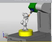
Test and confirm that every move inside your CNC is collision-free. Using Machine Simulation Pro to add machine components to your simulations, you're able to prove out position values, fixture locations and verify that your machine, table and fixtures have the necessary clearances to avoid potentially costly crashes.
